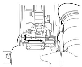
**3** Tighten the viewfinder forward-backward/left-right position clamp lever to the locked position.
